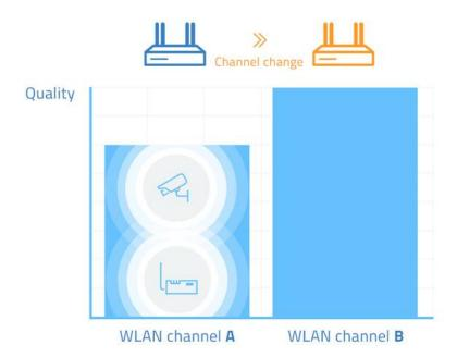
In LANconfig you have the option to manually configure the different thresholds that are used as the basis for an automatic channel change.
