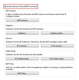
2. Configuring individual BGP instances: To configure the BGP instance of each router, click the BGP instance button
