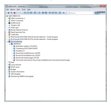
You also have the option to display the history of the connection tests. Click with the right mouse button on the entry **SLA monitoring**. In the following dialog, select **SLA monitoring history**.
