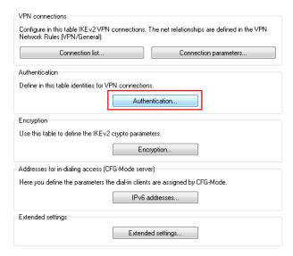
**4.** Click on the **Add** button to configure a new authentication type. Enter the information for the authentication of the VPN connection into the configuration window.
