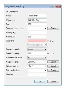
Give the neighbor a descriptive name and configure its IP address along with the number of the remote AS where it is located.
