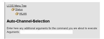
Specify a WLAN interface (e.g. WLAN-1) that should select a new channel and then click Execute.
