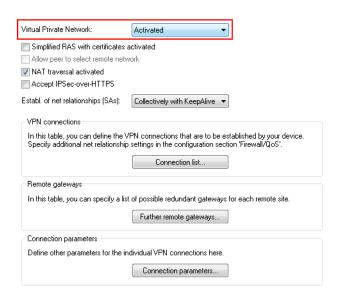
2. Configuration of the establishment of net relations (SAs): In order for net relations to be established correctly and according to the same schema, on each of the routers you should navigate to Establishment of net relations (SAs) and enable the option Collectively with KeepAlive.
