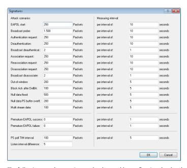
The following attack scenarios can be detected by configuring the thresholds and measuring intervals:
