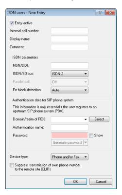
In the **ISDN parameters** section and under **ISDN/S0 bus**, select the option "ISDN 1 & ISDN 2" and then set the item **Parallel call** to "On".
