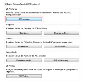
**3.** Use the configuration window to specify the general information about the BGP instance for each router. The screenshots below show the configurations for both devices for direct comparison side by side.
