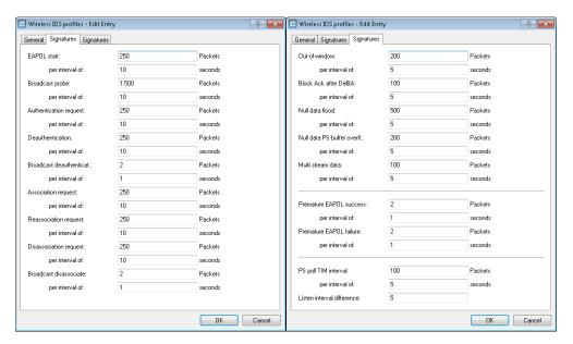
The following attack scenarios can be detected by configuring the thresholds and measuring intervals:
