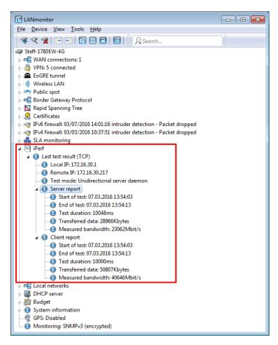
LANmonitor displays the test results stored in the device under **Status** > **Iperf** > **Last results**.
