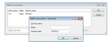
For SNMPv1 or SNMPv2c, you force the entry of login data for SNMP read-only access by disabling the public community in the list of the SNMP communities. This setting only allows information about the state of the device, current connections, reports, etc., to be read out via SNMP after the user authenticates at the device. Authorization can be conducted either with the administrator-account access credentials or an access account created for the individual SNMP community.
