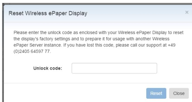
If a Display is reset after it was already associated with another Wireless ePaper Server, it must first be registered with the new server. Then it must be reset, deleted and registered again.
