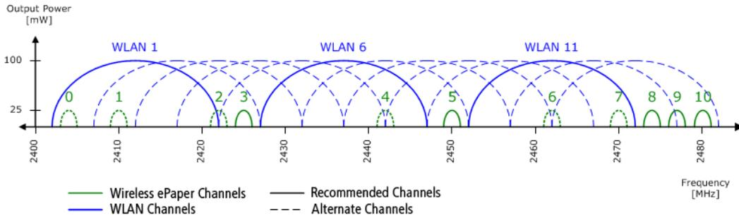
! Do not select the same channel for two access points that are in the same area. This causes interference and prevents Displays from joining the network. It is possible to set the same channel on two access points if you are sure that each display is only within range of one of these access points.
