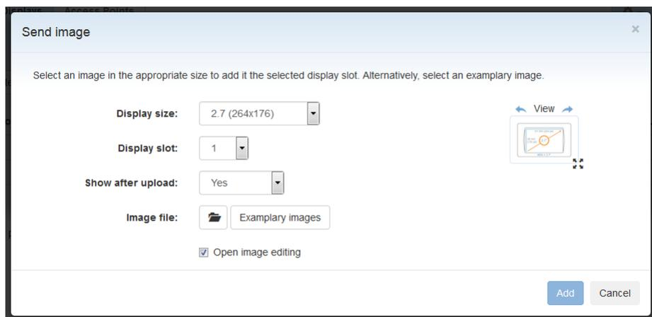
The display size is detected automatically. You select the desired image using "Image file (PNG, BMP)". LANCOM Wireless ePaper Displays support monochrome bitmaps in BMP or PNG format. The images need to have the same resolution as the Display. The image is displayed within approx. 10 seconds.
