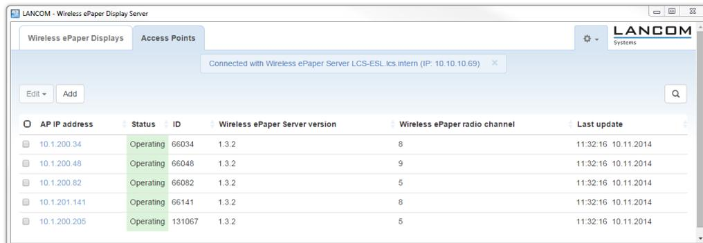
The screenshot shows the LANCOM Wireless ePaper Display Server management interface. The 'Access Points' tab is active, displaying a table of access points. The table has columns for AP IP address, Status, ID, Wireless ePaper Server version, Wireless ePaper radio channel, and Last update. All access points listed are in an 'Operating' status.
