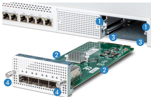
At first, power off your firewall with the power switch, and then disconnect the power cable from the device. Ensure to grant a potential equalization between yourself, the device, and the module during the complete mounting time.
