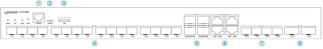
1 Configuration interfaces RJ-45 & micro USB (Console)
