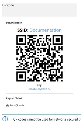
QR codes cannot be used for networks secured by 802.1X as they do not use a static WLAN key (PSK).
