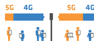
Fig. 5: Example of bandwidth allocation with Dynamic Spectrum Sharing (DSS)
