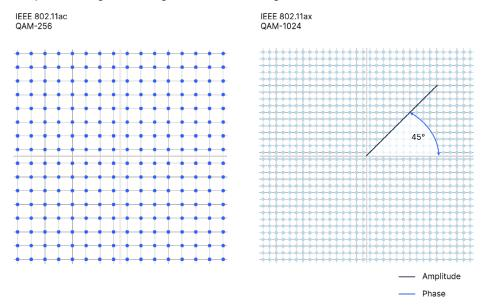
Figure 5: QAM-256 vs. QAM-1024
