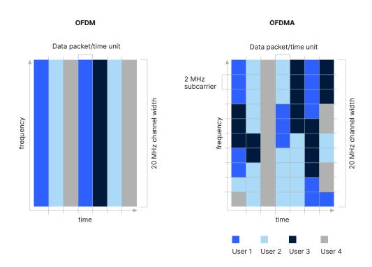
Figure 3: Comparing OFDM (Wi-Fi 5) vs. OFDMA (Wi-Fi 6) technologies
