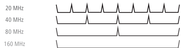
Fig. 1: Possible channel bandwidths with Wi-Fi 6
