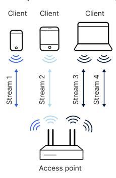
Figure 2: Multi-User MIMO for down- and uplink
