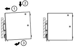
Snap the power supply unit onto the DIN rail as shown:
