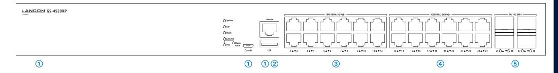
Configuration interfaces RJ-45 & micro USB (Console) Connect the configuration interface via the included micro USB cable to the USB interface of the device you want to use for configuring / monitoring the switch. Alternatively, use the RJ-45 interface with the provided serial configuration cable.
