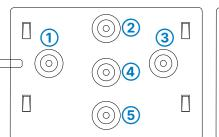
Use the supplied screws to fix the back plate to the wall using the holes (1), (3), and (5).
