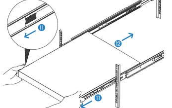
Now move both of the blue plastic sliders at the inner rails on each side of the device to the front (1), and simultaneously push the device into the rack until it is noticeably locked in its end position 😰.
