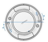
The screws **C** are now locked in their end positions **5** and the access point is fixed to the mounting plate.
