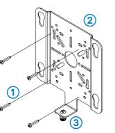
Depending on the wall material structure, select 4 suitable pan head screws M4×35 (1) and, if necessary, suitable dowels for mounting the retaining plate (2) on a sufficiently load-bearing
