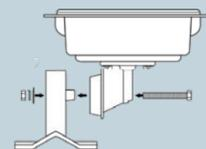
The main beam direction of the integrated antenna can be adjusted by tilting the access point up or down by rotating the connection flange about the mounting arm.
