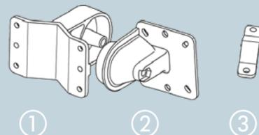
Screw the connector flange ② to the back of the housing with the four screws and their washers.
