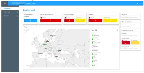
The web-based LANCOM R&S®UF Command Center is the ideal solution for managed-security service providers and companies that need to centrally manage, configure, and monitor large numbers of LANCOM R&S®Unified Firewalls. An intuitive dashboard enables management and monitoring, centralized backup administration and archiving as well as license monitoring of all managed LANCOM R&S®Unified Firewalls.
