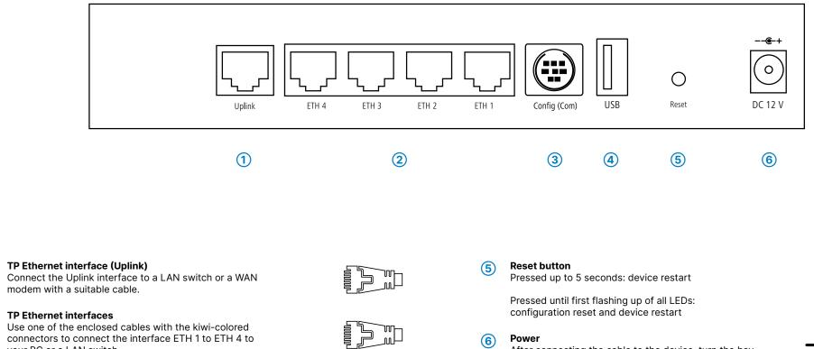
Use one of the enclosed cables with the kiwi-colored connectors to connect the interface ETH 1 to ETH 4 to your PC or a LAN switch.
