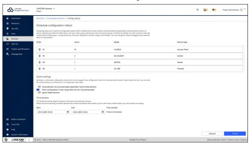
Configuration rollouts and firmware updates can now be planned in advance and executed automatically, eliminating the need for active administrator involvement. All that is required is to define the time window and select the respective devices beforehand.
