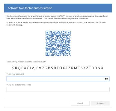
Two-factor authentication secures your LMC access. Besides your password, you will be asked for an additional factor. This factor is a time-based one-time password based on RFC-6238, using a 160-bit key.
