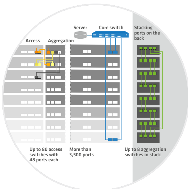
Fig. 11: Detailed view of up to eight LANCOM XS-6128QF in ring-topology stacking
