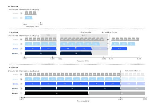
Figure 1: Frequency scheme 2.4 GHz, 5 GHz, and 6 GHz
