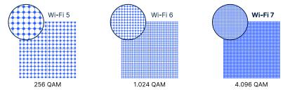
Figure 3: QAM (quadrature amplitude modulation)
