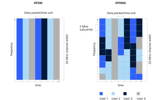
Figure 1: OFDM (Wi-Fi 5) compared with OFDMA (Wi-Fi 6) technology
