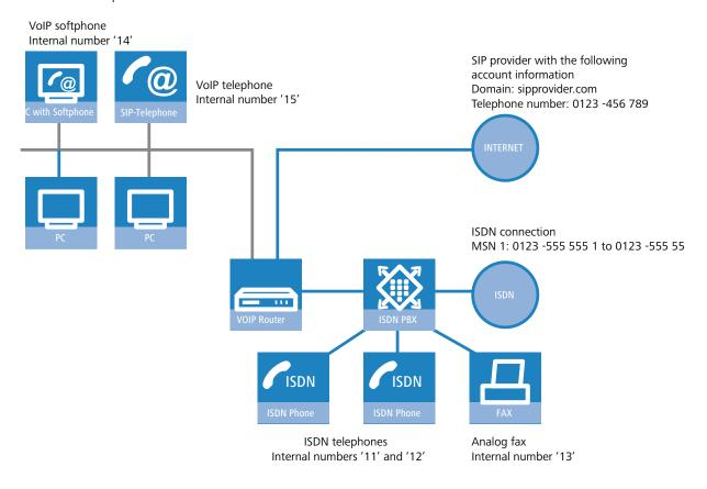
The LANCOM is operated on an ISDN PBX extension line.
