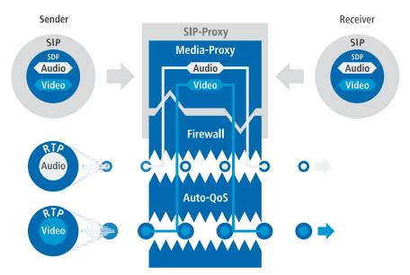
All of the connection information in the direction of the SIP provider can be maintained and all of the necessary changes to IP addresses, ports, etc., are handled by the media proxy.
