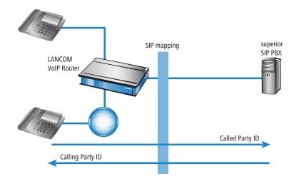
SIP mapping is configured under **Voice Call Manager** > **Lines** by clicking the button **SIP mapping**.
