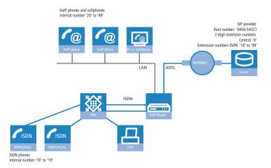
In this example we will take a look at a company planning to add a SIP trunking account with up to 10 extension numbers. The ISDN terminal devices with point-to-point line extensions used thus far can be retained. All new employees are to be issued with a SIP telephone with an extension via the SIP account.
