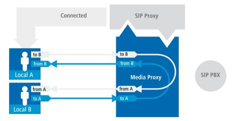
In this case it is not necessary to pass the media streams through the upstream PBX, so the SIP signaling helps the LANCOM VoIP router to make a new decision about the path to be taken by the connection data. Using the end points in the media proxy the data streams can be connected directly, making a diversion via the SIP PBX unnecessary.
