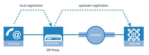
The great advantage with this two-stage registration comes to bear in the backup event: If the connection to an upstream SIP PBX is not available, the SIP proxy can handle the user who is registered upstream as a local user and can then direct the calls over alternative lines.
