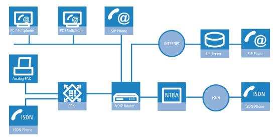
Telephone calls over the PBX and its ISDN telephones remain possible just as before; the telephones remain available under the familiar telephone numbers. This application additionally offers the following options:
