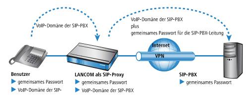
If SIP or ISDN users at the LANCOM VoIP router are entered into the SIP PBX with different passwords, then the users have to enter their individual passwords upon registration. Consequently, each SIP or ISDN user has an entry in the
