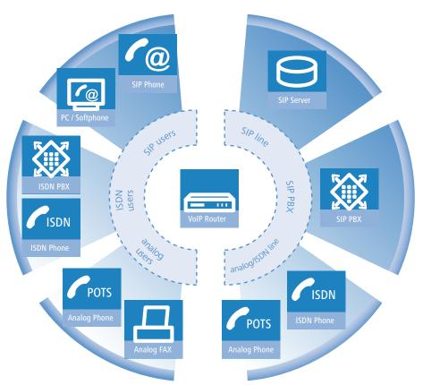
6. The external ISDN world via ISDN NTBA or upstream ISDN PBX, and all of the external subscribers available via the land-line network
