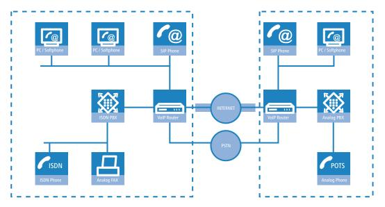
Along with data transfer via VPN, it is also possible to use VoIP functions between the two locations.
