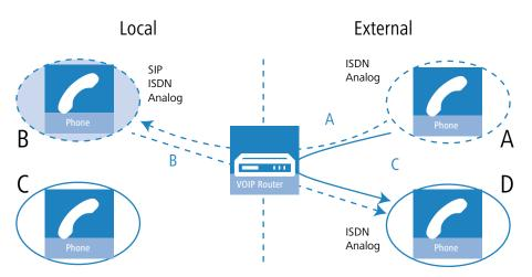
5. If both external users **A** and **D** use SIP, the LANCOM VoIP router is unable to forward the call.
