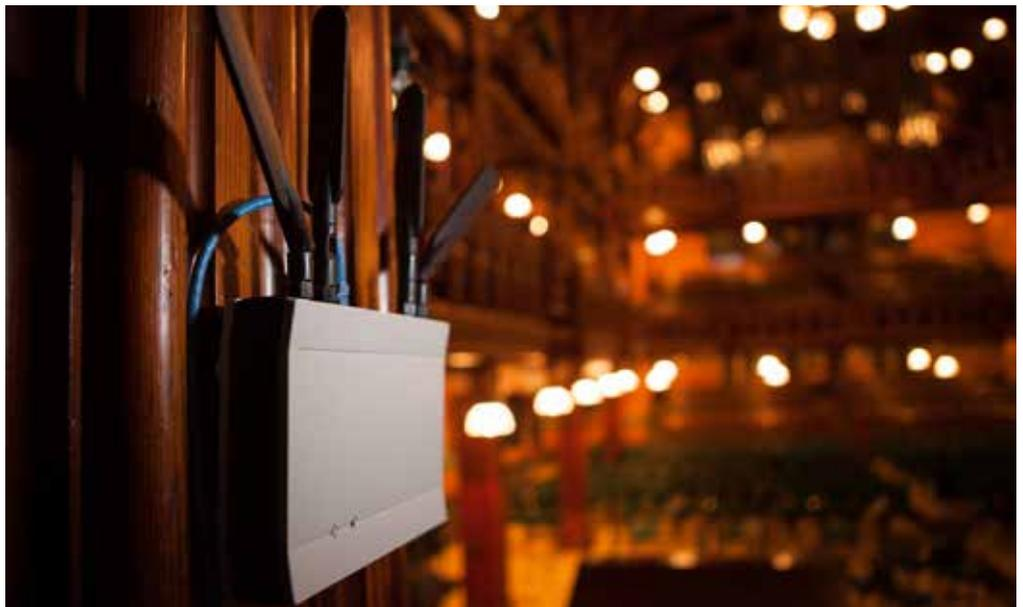
The access points are managed centrally by two LANCOM WLC-4100 controllers. These effectively implement three different networks across the same infrastructure using a system of service set identifiers (SSIDs). These assign different filters and access rights to different user groups. Each SSID defines a user profile that can be set up on the controller, which then configures all the associated access points remotely.
