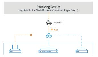
Principle of the Open Notification Interface: A device goes offline -> the notification is created in the LMC -> the LMC notifies the external receiving service.
