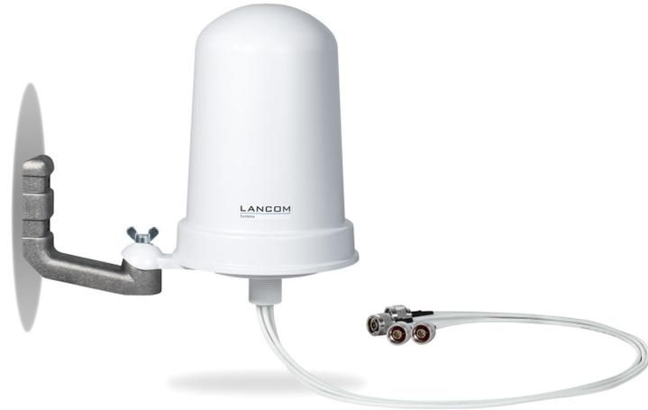
The weatherproof LANCOM AirLancer ON-Q360ag omni-directional antenna provides effective WLAN over wide areas. Mounted centrally, it is ideal for 360° coverage. Thanks to 4x4 MIMO, it offers maximum performance for the WLAN standard IEEE 802.11ac. It is ideal in combination with dual-radio access points to offer parallel operation at 5 GHz with 2x2 MIMO and 2.4 GHz with 2x2 MIMO.
