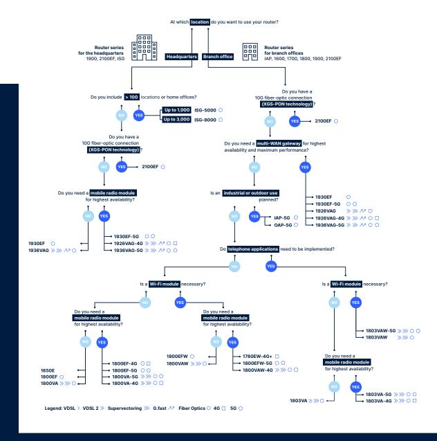
For projects that require the integration of <u>professional telephony functions</u>, we recommend the LANCOM 2100EF, the 1900 series, and the <u>LANCOM VolP routers</u>. All LANCOM gateways and routers can be further upgraded with various <u>software options</u>, e. g. with an All-IP function, a content or BPjM filter, additional VPN channels, and much more.
